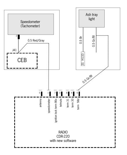
Work Procedure: **2.3** Attach the connector, part number **N 903 352 04** to the end of the Gray/Blue wire and insert into plug K14 in the Central Electric Board.
